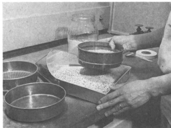
FIG. 2.—An 8-week-old culture of lesser grain borer is being screened by hand with a U.S. Standard Sieve no. 10; a no. 20 sieve is used next to separate dust from the insects.
